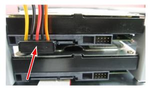
3. Place the HDDs inside the DVR, screw the HDDs from the bottom side of the DVR using the supplied Screws. After installing the HDDs, screw the housing cover back to the DVR.
