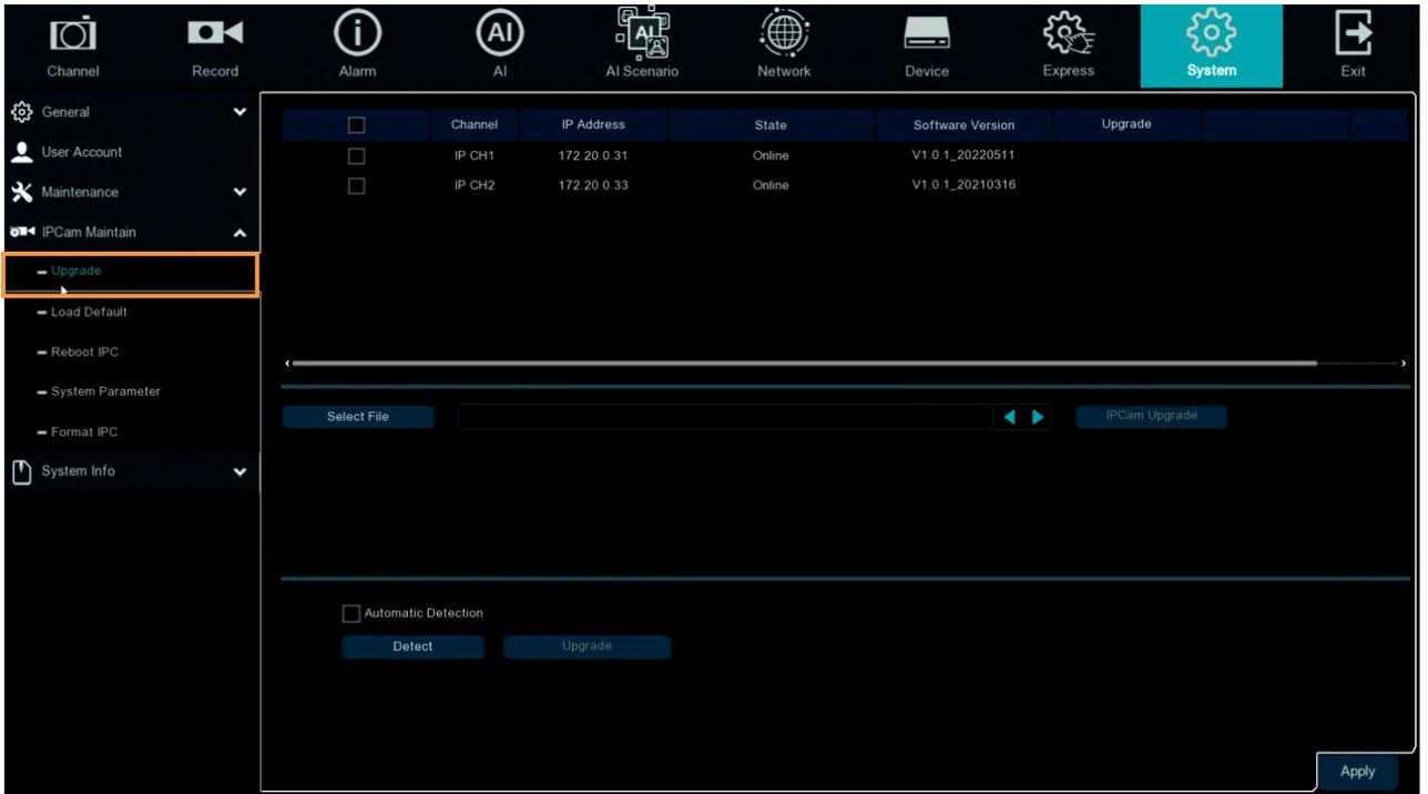
1. Select one of the IP cameras you want to upgrade firmware by checking the checkbox.
