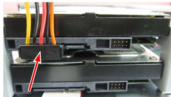
4. Place the HDDs inside the XVR, screw the HDDs from the bottom side of the XVR using the supplied Screws.
