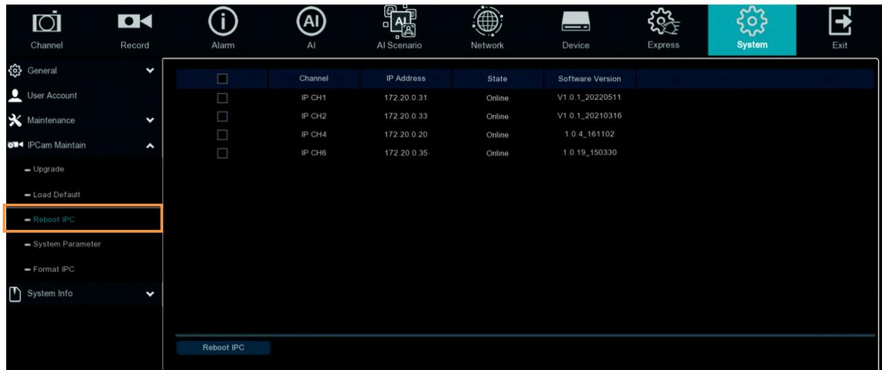
1. Select one of the IP cameras you want to reboot by checking the checkbox.
