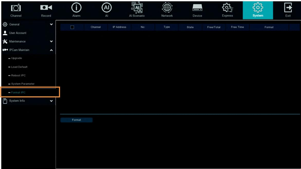
This function can detect SD memory card connected to an IPC with the API protocol, and Click Format's SD card for the IPC that can be formatted.
