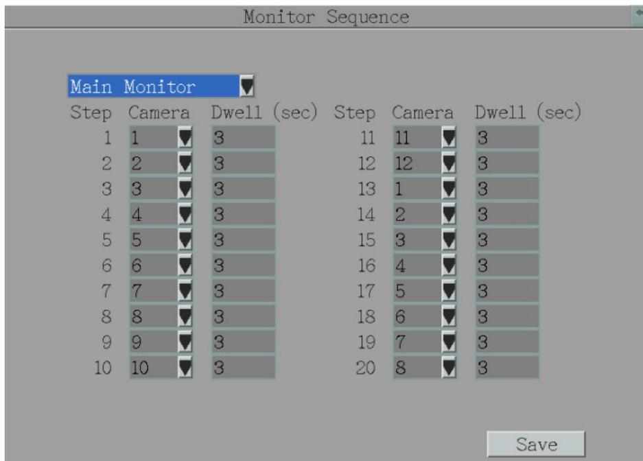
**Monitor Drop-Down:** Select Main Monitor or Call Monitor for setting up the below parameters.
