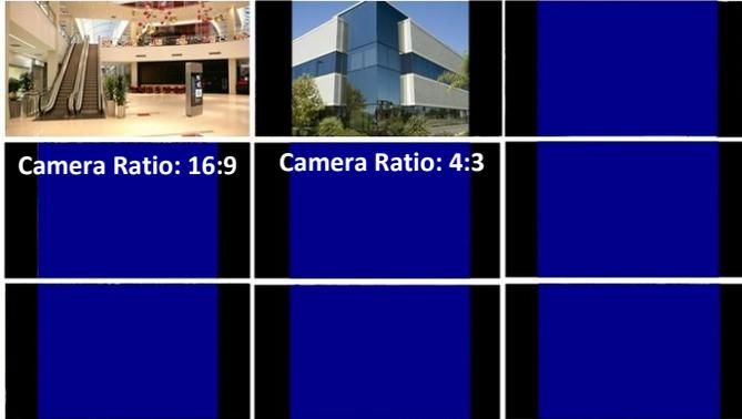
If you select 800x600, 1024x768 or 1280x1024 (4:3) screen resolution on the **Screen Mode** drop-down list (see 6.5.1 *Monitor OSD*), it is recommended to also change the camera live view display to 4:3 aspect ratio on the **Ratio** drop-down list (see 6.1.1 *Analog Camera*).
