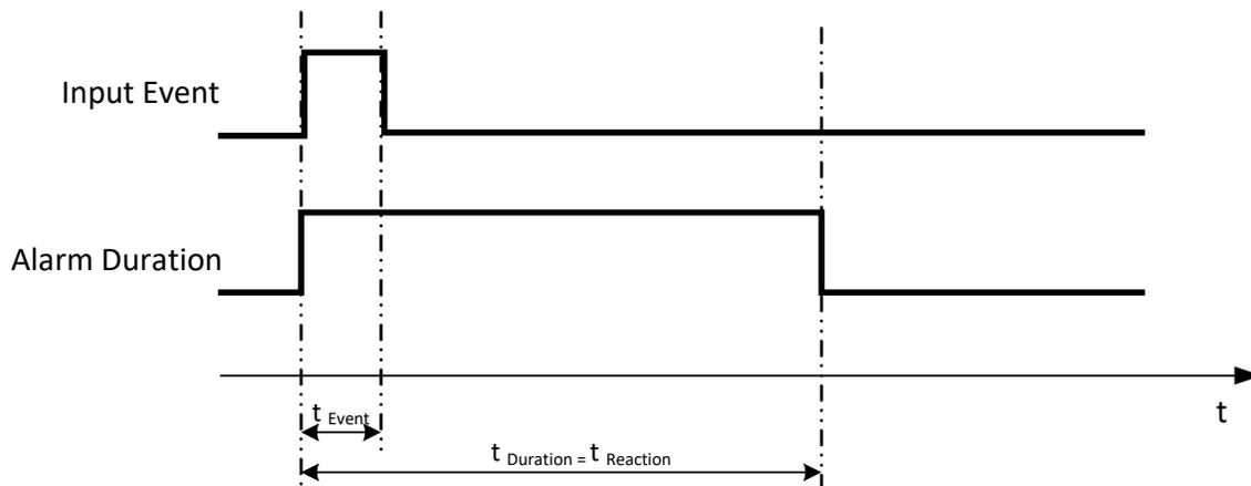
**$t_{\text{Event}}$ :** Duration of alarm input source (contact, system events...)
