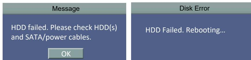
Note that the DVR/MDVR will automatically reboot to detect HDDs up to 3 times. If the Auto HDD Retry process exceeds 3 times and the DVR still cannot detect HDDs, an *“Auto HDD Retry exceeds 3 times.”* message will pop-up and a continuous beep sound will be played for notification. It’s recommended to check the SATA and power cables connected to the HDDs; or replace new HDDs if necessary.
