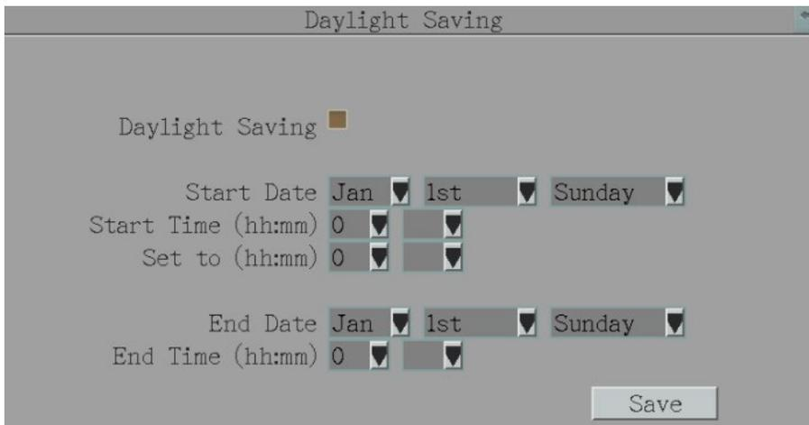
**Daylight Saving:** Check the box to enable automatic daylight saving time (DST).
