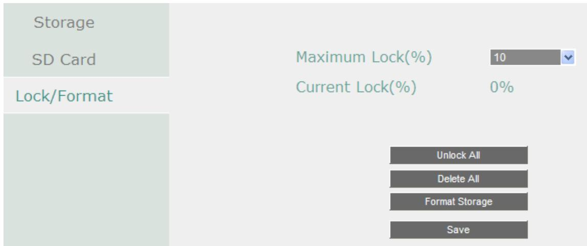
**Maximum Lock (%):** Sets the maximum percentage of the hard disk space reserved for Locked Event Recordings. To set up the Locked Event Recordings, please select the **Auto Lock** item in *7.3.1.1 Alarm*.
