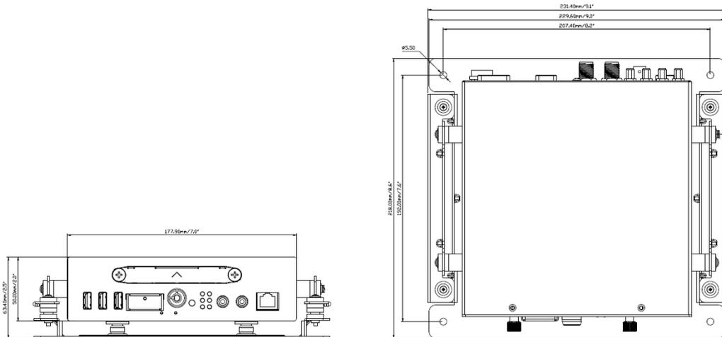
**Installation:** The **Bracket** is already installed on the mobile DVR. To mount the mobile DVR onto a surface, use the supplied 4 black screws and 8 spacers (place 2 spacers on each screw hole).
