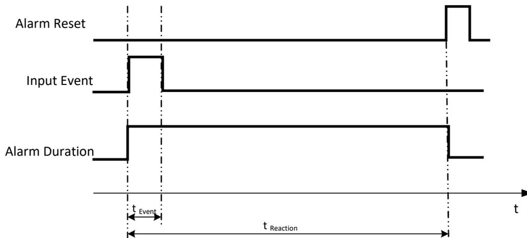
**$t_{\text{Event}}$ :** Duration of alarm input source (contact, system events...)
