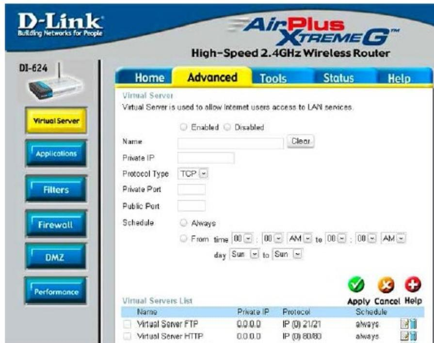
Virtual Servers allows users who are connecting remotely to access services on the router's Local Network. The functions of each field are described below.
