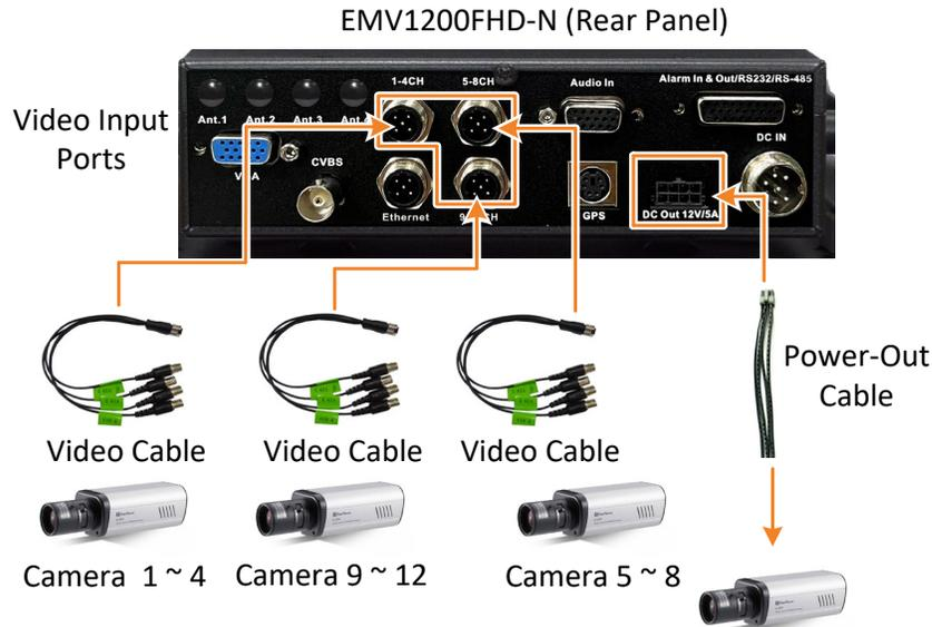
You can also use the supplied Power-Out Cable to power on the connected cameras. The Power-Out Cable provides four set of power output wires (+/-). A total of 12VDC, 5A power output is provided. You can optionally prepare the wires and connect the wires to the Power-Out pins for powering up more cameras.
