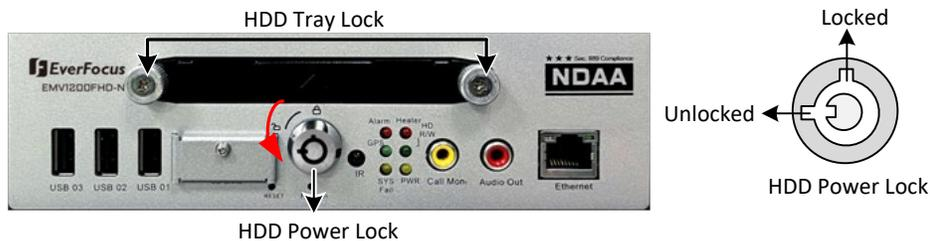
2. Insert a HDD in the HDD Tray and then screw the HDD to the tray with the supplied 4 screws.
