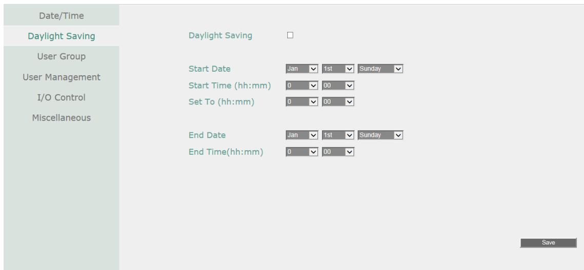
**Daylight Saving:** Check the box to enable automatic daylight saving time (DST).
