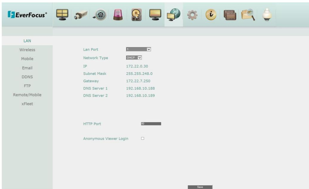
**LAN Port:** The mobile DVR supports WAN and LAN network connections. Select **1** (WAN) or **2** (LAN) from the drop down list and further set up the below network settings.
