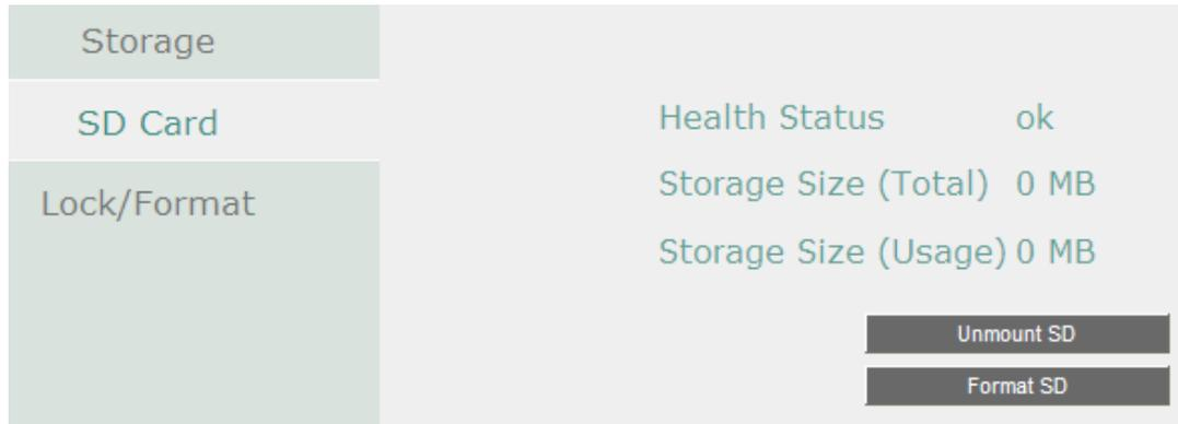
**Unmount SD:** Before removing the SD card from the mobile DVR, please click the **Unmount SD** button first for data safety purpose.
