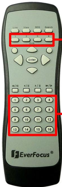
**MDVR Device Number:** The ID number here must correspond to the “IR Remote ID” in “I/O Control Setup Menu”. The buttons are used to select a mobile DVR when there is more than one unit. Selecting an incorrect unit ID will prevent the mobile DVR from responding to commands from the remote.
