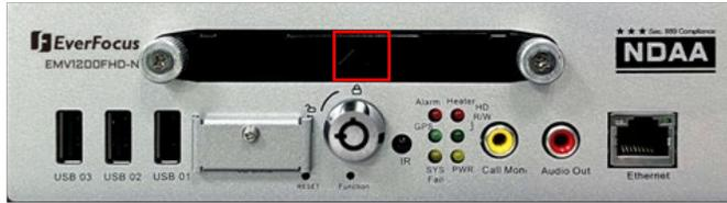
4. Lock the **HDD Tray Lock** and **HDD Power Lock** before you power on the mobile DVR.
