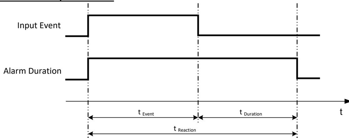
**t<sub>Event</sub>**: Duration of alarm input source (contact, system events...)
