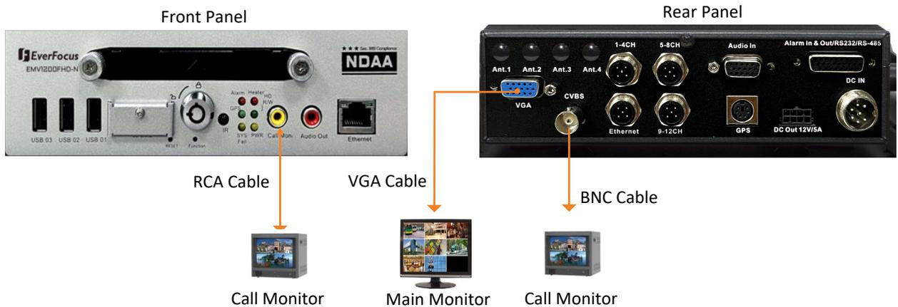
You can also optionally switch the RCA / BNC video output from call monitor to main monitor; and mean while, switch the VGA video output from main monitor to call monitor. To do this, press the **Function Key** on the front panel for 3 seconds, the system will start rebooting. Once the system reboot process is complete, the Main and Call monitors will be switched (see image below). To switch back the main and call monitors, press the button for 3 seconds again.
