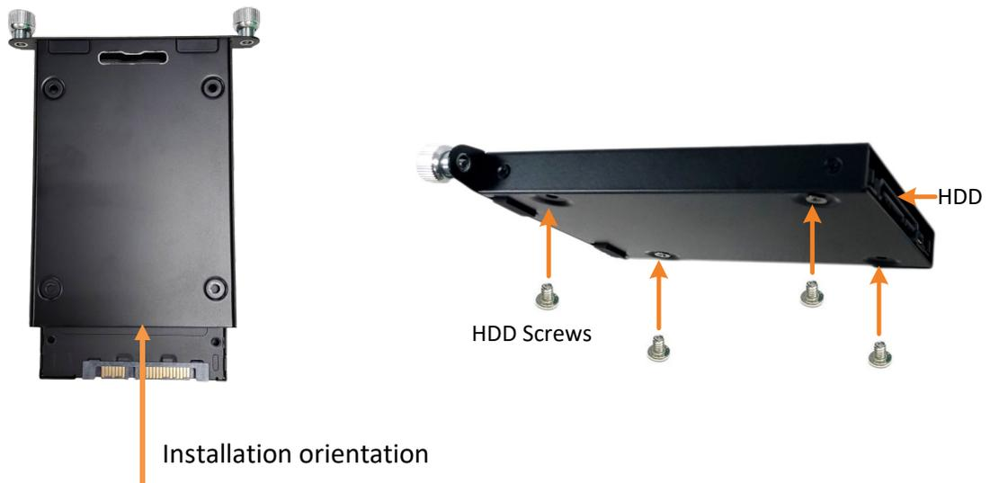
3. Insert the HDD Tray into the drive bay and close the **Locking Arm**. Please place it in the correct orientation according to the arrow direction.
