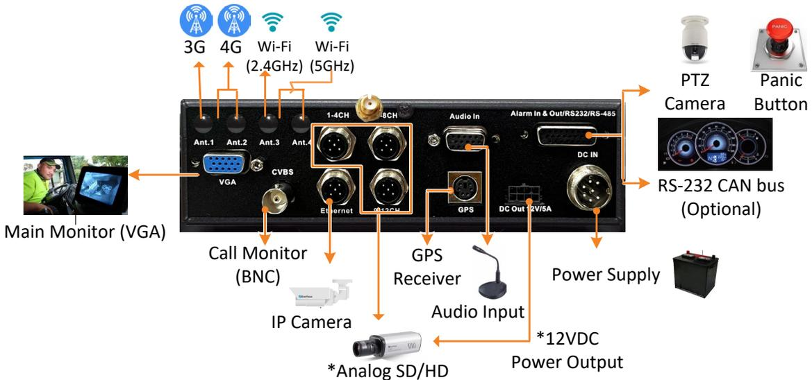
\* The EMV800FHD-N / EMV1200FHD-N have 4 power output sets (+/-) to power-up the connected cameras. A total of 12VDC, 5A power output is provided. Please refer to *2.5.2 Video Cable / Power-Out Cable* for more details.
