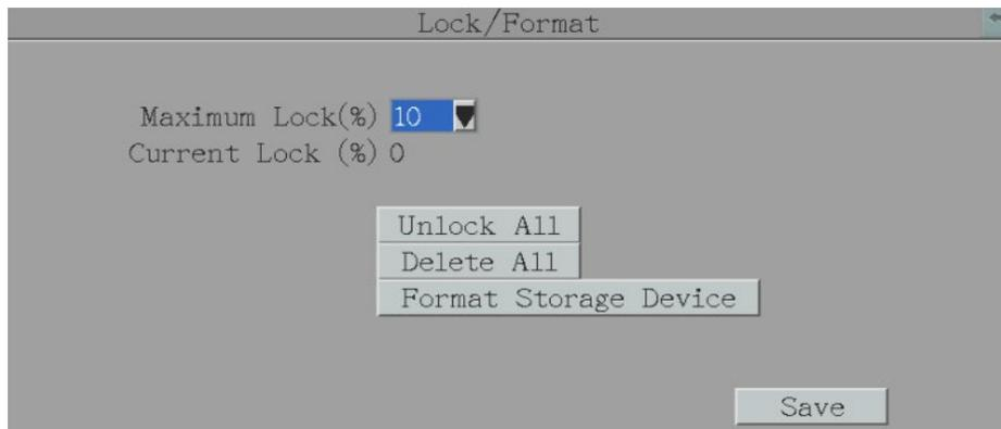
**Maximum Lock (%):** Sets the maximum percentage of the hard disk space reserved for Locked Event Recordings. To set up the Locked Event Recordings, please select the **Auto Lock** item in *6.3.1 Alarm*.
