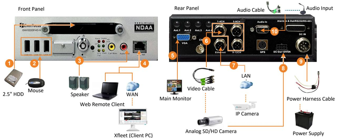
1. To record videos, insert a 2.5" HDD (or SSD) to the HDD tray. Remember to lock the HDD Key Lock after inserting the HDD or the recording will not start (see 2.2 Hard Disk Installation).
