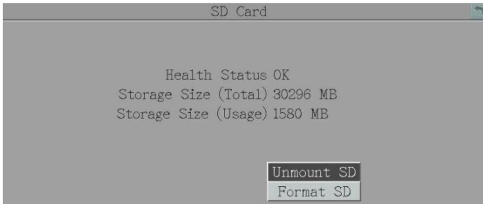
**Unmount SD:** Before removing the SD card from the mobile DVR, please click the **Unmount SD** button first for data safety purpose.
