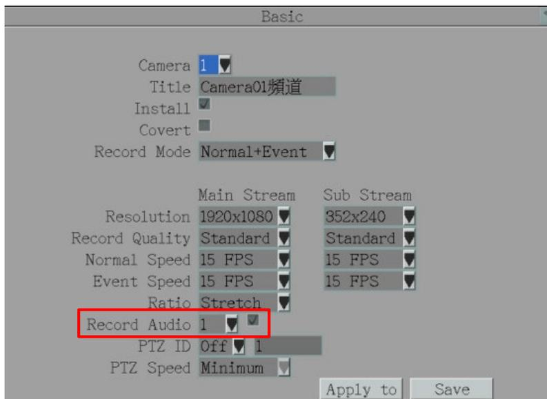
Note that the mobile DVR only provide one channel audio output. You can switch the Audio Output function to either one from the cameras. To switch the Audio Output function to the desired camera:
