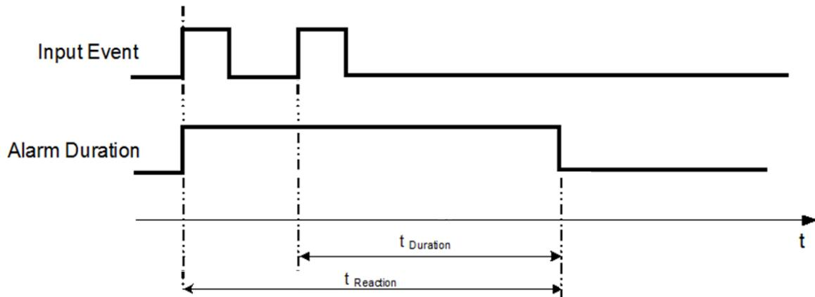
**t<sub>Event</sub>:** Duration of alarm input source (contact, system events...)
